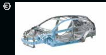
Energy Absorbing Body Structure & High Strength Body Frame (semua tipe).
